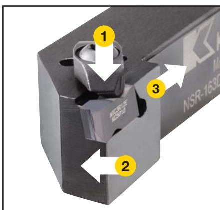
Our rigid clamping design prevents insert movement during high-feed rate applications. This benefit ensures excellent surface finish, improved productivity, and superior tool life and promotes perfect concentricity. The rugged bridge clamp generates locking forces in three directions to provide superior resistance to side thrust and tangential forces.
