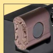
Modified cartridge with approach angle of 93° (difference of 6°)
