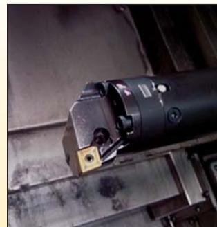
Figure 3: Boring bar collar flat
