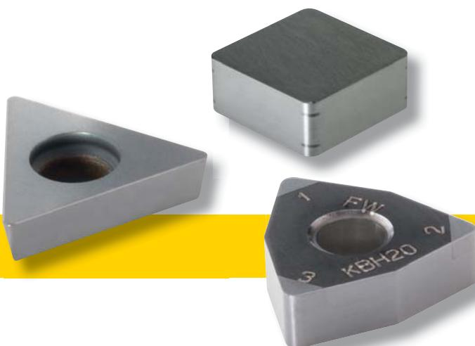
PcbN is thermally stable up to approximately 1200° C and has high resistance to chemical attack. As a result, extreme temperatures like those that occur when machining hard ferrous metals do not cause difficulties and can be used to promote self-induced hot cutting. This adds technical and productivity benefits, especially when compared with grinding. In most cases, performance is significantly better than that attained with conventional tool materials, such as tungsten carbides and ceramics.
