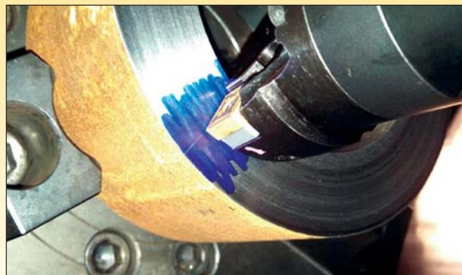
Figure 5: Boring bar centre height
