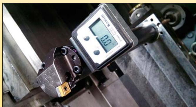
Figure 4: Aligning the boring bar
